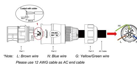
3. Plug the AC port Part 2 into Part 1 once complete the wiring, and screw the Part 3 on and complete the AC extension cable:
